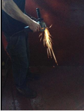
Wrought Iron : Short train of straight orange sparks that burst with no feathers.
