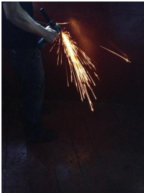
H13 (tool steel) : Shorter length sparks than EN9 Same colours with bursts and little feathering.
